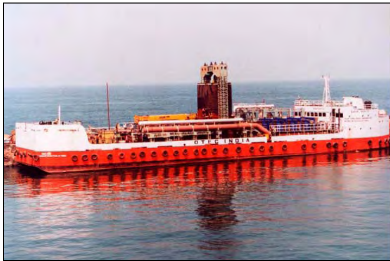
Figure 7-43: India 1 MW Floating OTEC Pilot Plant
