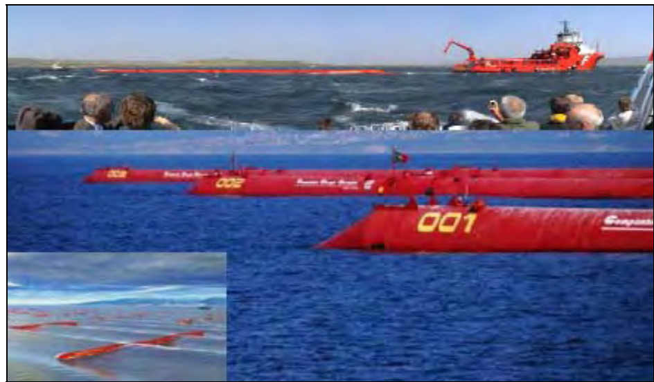
Figure 7-29: Pelamis – Three 750 kW machines in Portugal
