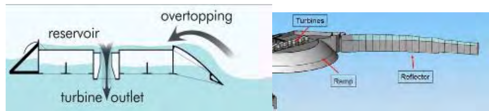
Figure 7-36: The basic principle of the Wave Dragon
